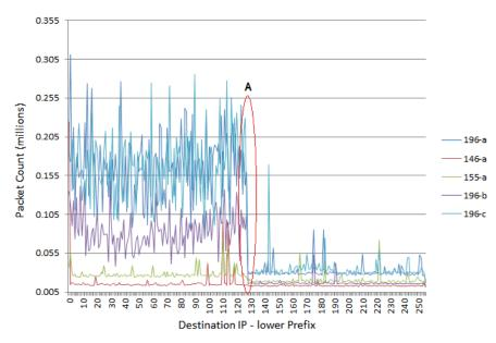
Figure H.1: Packet distribution across destination IP for all network telescope sensors
