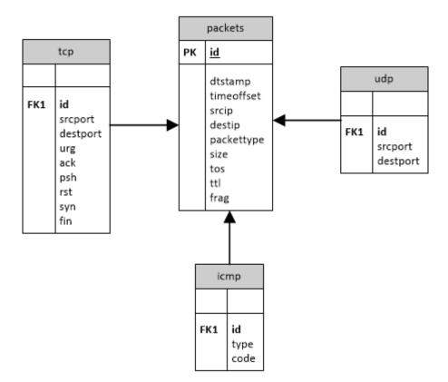
Figure 3.2: Entity relationship diagram of database schema
