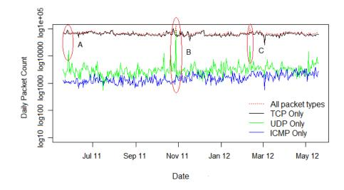
Figure 4.5: Daily packet count of telescope sensor 196-c between 20 May 2011 and 20 May 2012 - protocol overview
